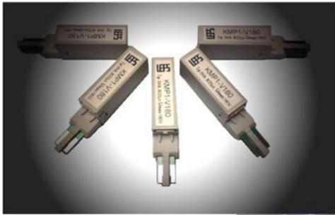
Quick and easy plug-in installation -The KMP series protectors can be easily plugged into the KRONE LSA-PLUS disconnection blocks and are earthed via the earth bar to the back-mount frame.
